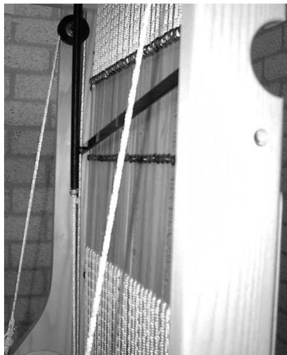
The rest position of the knife has to be adjusted so that the screw head of the last shaft can freely move under the knife. Place the eye bolt in its proper height and tighten by turning the nut and knurled nut in opposite direction so they tighten in the large hole.
