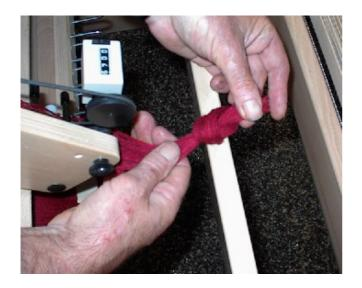
Put a knot in the end of the warp that sticks out of the warp tension regulator.
