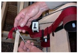
Take a tie-up cord and attach this with a lark's head onto the tie-up rod. Connect the other end of the tie-up cord to the warp also with a lark's head behind the knot in the warp yarns.
