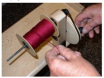
For every thread in the section you need a bobbin on the bobbin rack. With the bobbin rack you can have a maximum of 16 threads per cm with metric beams. If you have an imperial beam you need to replace the metric raddle with the imperial one, in which case you can have 32 threads per inch on one bobbin rack.
