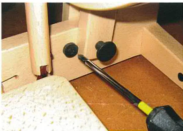
If it happens that some play arises in the locking system of the post, it can be repaired by adjusting the buffer. Release the screw of the buffer and turn it to a position so that it pushes the bottom of the post slightly backwards. The locking knob should fall inside just when the post hits the buffer. Fasten the screw after the buffer is turned into its proper position.
