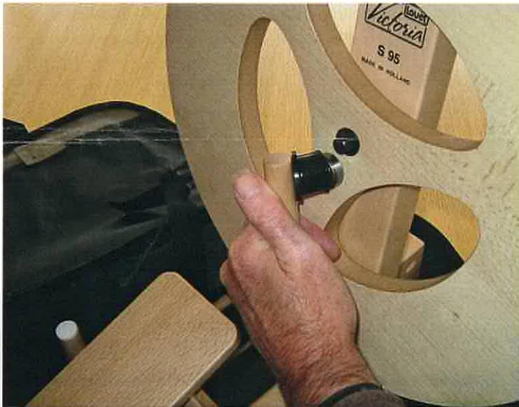
Place the cup on the footman over the ball bearing of the wheel and push the locking ring forward against the rim on the cup. If you position the cup at an angle to the bearing, while pushing it on, the cup snaps on easier. When you need to remove the cup again, the proper technique is to twist the footman, allowing the cup to snap off of the bearing.
