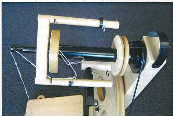
Put the drive band in one of the three grooves of the pulley. The largest diameter has a 1:6 ratio, and you will get fewer twists per inch with the same treadling speed compared to a higher ratio.
