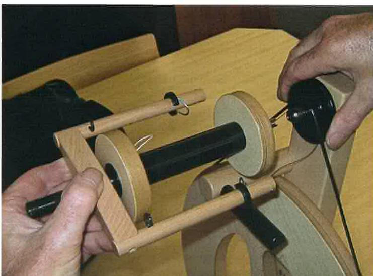
Place the brake band in the groove of the bobbin and guide it around the hook. Turning the black knob tightens the brake band around the bobbin end. You can see the brake tension increase when the spring expands. If you need to, you can adjust the friction of the knob by turning the screw that holds the knob.
