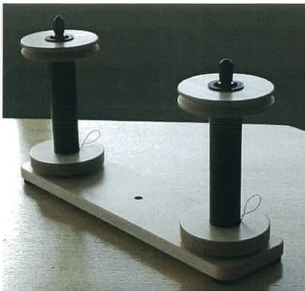
The lazy kate has an extra hole in the middle. An axle for a third bobbin will fit in this hole.
