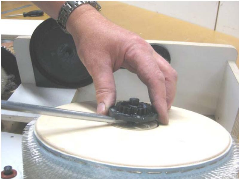
Remove the tooth wheel. If it is hard to do, use a tool like a flat head screwdriver.
