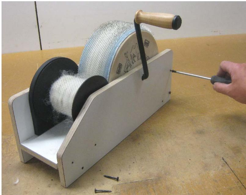
Unscrew the four screws that hold the frame side.
