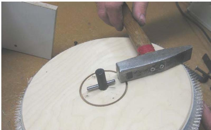
Tap the locking pin out of the axle.
