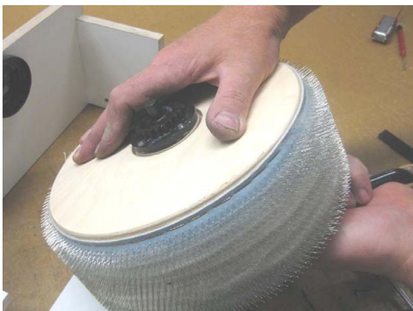
Press the drum towards the frame side, while turning the crank a bit.
