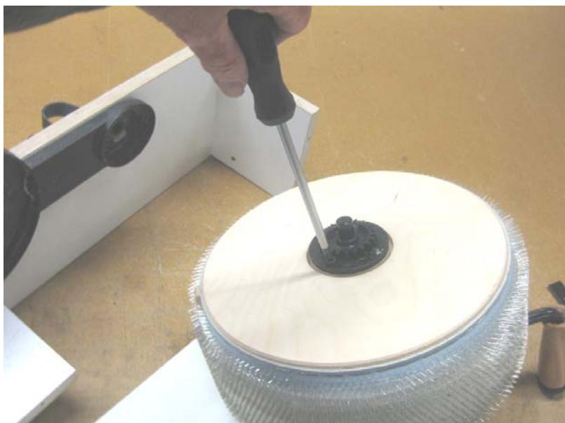
Unscrew the four screws that connect the tooth wheel to the drum side.
