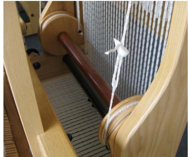
Lead the cord one and a half times around the disc (mirror the cord on the disc on the other side) and connect both ends of the cord as shown in the picture.
