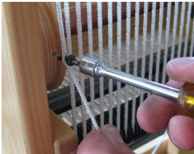
Pull the end of the cord along the disc to determine the cord loop that corresponds to the screw hole in the disc.
