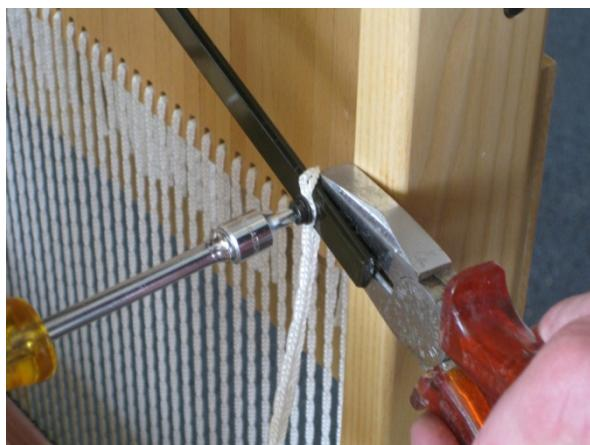
Fasten the bolt with the nut into the hole in the knife. The cross head of the little bolt is Philips head and does not match the pz2 screwdriver that was supplied with the loom.
