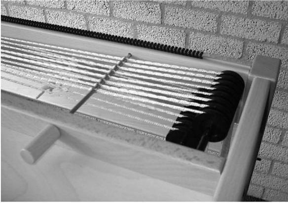
Insert the locking pin into the hole in the top rail and through the marked cord loops. Now the shaft bars and lams are fixed in their neutral position.
