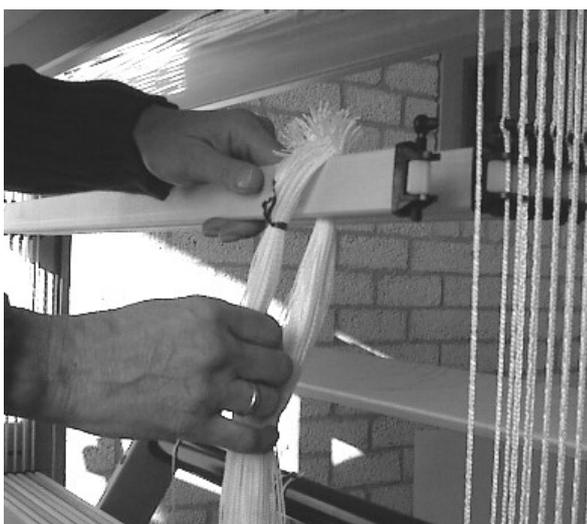
If you need to add heddles to a shaft, pull the hook that connects the upper shaft bar to the cord, out of its cord loop. Slip over a bundle of heddles and push the hook back into the same loop again. Repeat this with the lower shaft bar, but untie the bundle before you attach the lower bar into the cord again.
