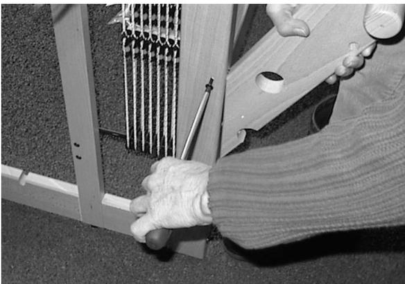
Secure the polyurethane dowels by screwing the screws completely into the uprights, while holding the back part in a position that lets the dowel in completely.
