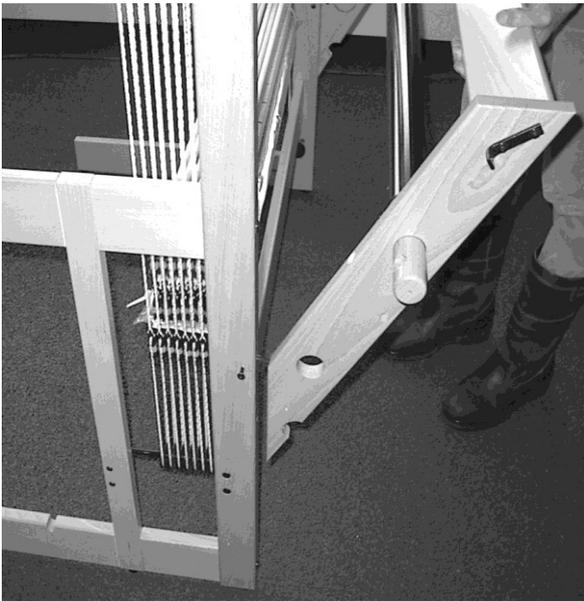
Place the back part in its location by inserting the polyurethane dowels into the holes at the rear of the loom.
