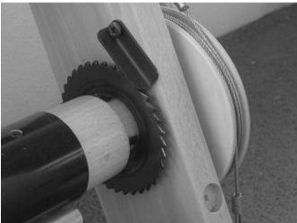
Screw the pawl into the hole above the ratchet wheel. Then again a little loose, so that the pawl can rotate. Put the pawl out of the ratchet wheel during the weaving and use of the brake like the picture shows. When putting a warp on, it is convenient to use the ratchet wheel and release or take off the brake cable.
