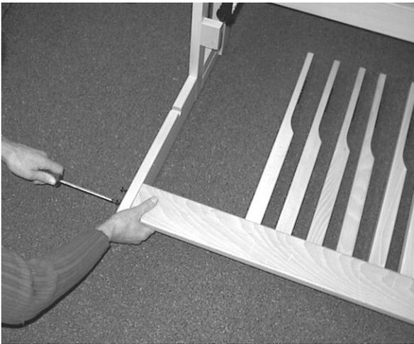
Turn the foot rail right side up again around the axles of the treadles, while the treadles stay on the floor and connect it with the four remaining screws to the base side pieces.
