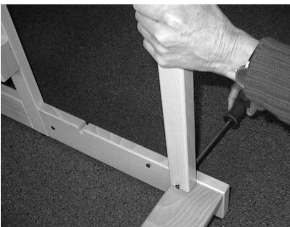
Screw four of the small screws into the pilot holes at both sides at the bottom of the floating arms and a small screw at the inside of the base side pieces. The heads of these six screws have to protrude about 5 mm (3/16").
