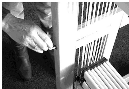
Fasten the side parts with the socket-head screw wrench.
