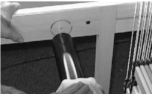
Install the cloth beam with the wooden end into the hole of the right middle side piece and the metal end into the circular groove of the left side piece. You will need to push the side pieces apart to install the cloth beam in between.
