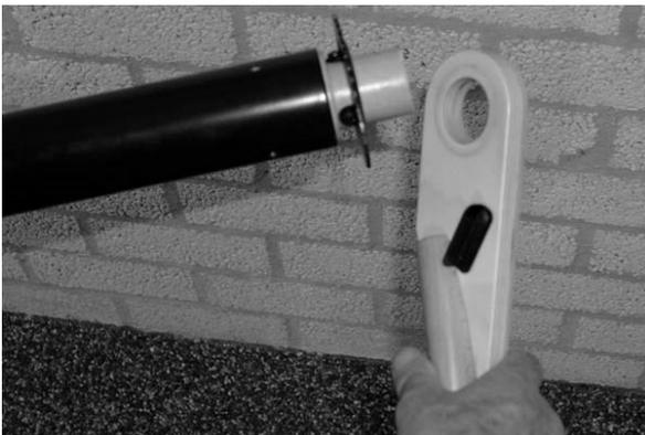
Slide the cloth beam lever onto the cloth beam and make sure that the ratchet is on the right side of the ratchet wheel.
