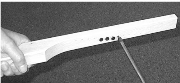
Screw the small screws into eight holes of each treadle, so far that the screw heads protrude approximately 5 mm (3/16") from the wood. The thread of the screws should just disappear into the wood. Use the eight holes closest to the end of the treadle; the other four holes are to be used for an extension to twelve shafts.
