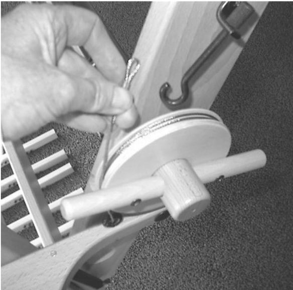
Attach the threaded hook and the knurled nut to the bracket as shown on the picture.
