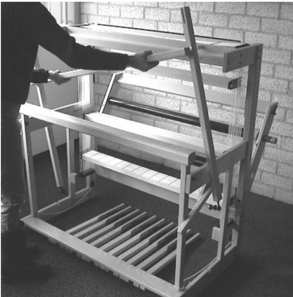
Place the assembly of uprights and lower reed tray into the loom. First guide one hinge along the side rail and then the other one. Put the hinges into the openings in the base side pieces.
