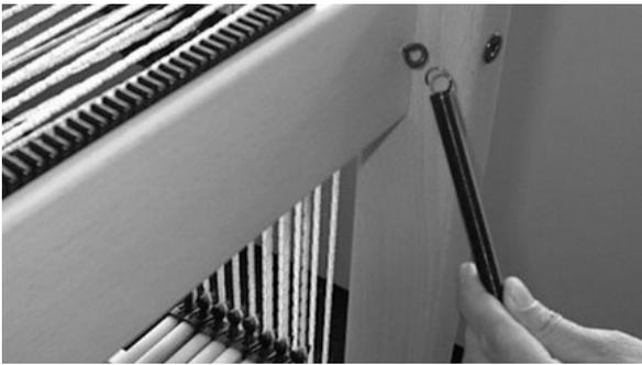
Hook on the springs to the screw eyes on the back at the top of the middle part.
