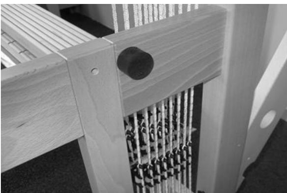
Screw the buffers into the holes at the sides of the loom, see picture. If your loom has twelve shafts you need to use the other hole you see on the picture.
