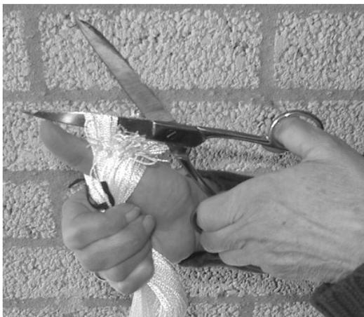
Cut with sharp scissors at the ends of the bundle of heddles the loops with which the heddles are connected to each other. Only remove the straps from the bundles after the shaft bars have been inserted, otherwise a big mess will occur
