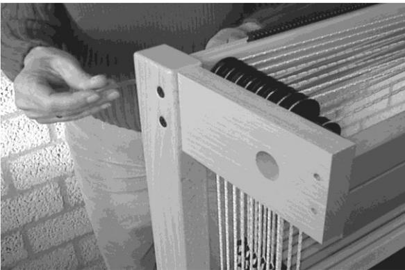
Unscrew the socket-head nut and remove the side piece. If the threaded end remained in the barrel, take it out and take the barrel nut out too.
