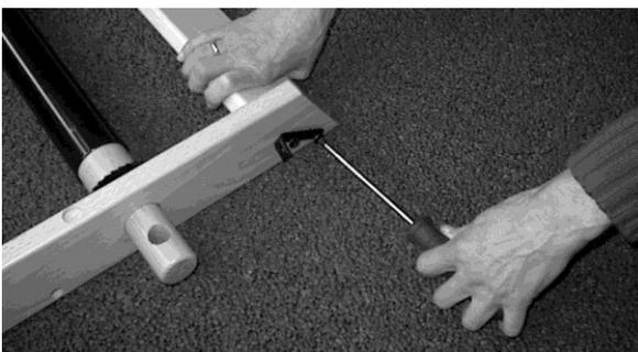
Attach the supports to the back beam with the remaining 50 mm screws. At the right side you have to use these screws to attach the metal bracket.
