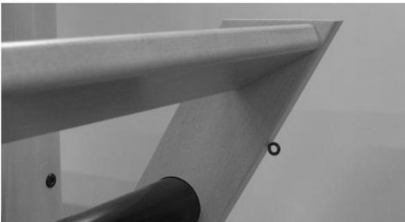
Screw the two screw eyes into the pilot holes at the backside of the warp beam supports. If you are used to leaving the lease sticks in the warp, attach them to these eyelets.
