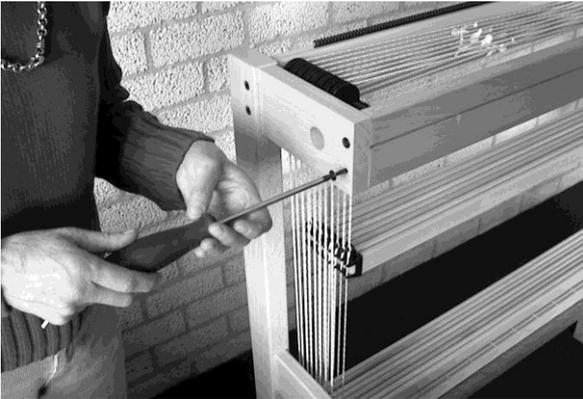
It is important that the axles with rollers stay between the front and back rail. This means the front rail needs to be pushed backwards while replacing the side pieces. Make sure you replace the side pieces one by one!
