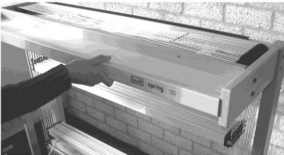
Place the front rail of the shelf. Make sure the shelf bottom slides into the groove.
