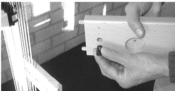
Insert the barrel nuts into the holes of the side pieces.
