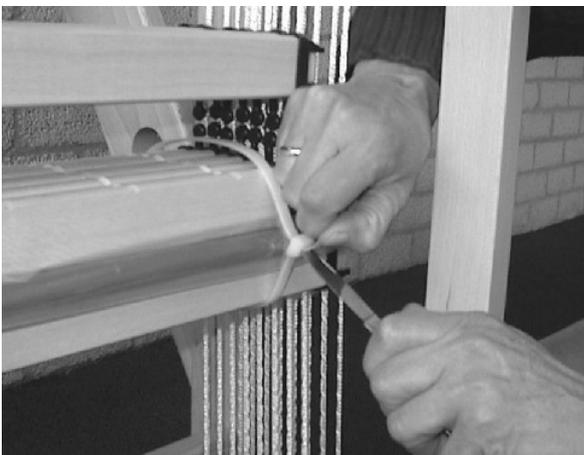
Remove the reed from its location between the lambs by taking away the tie straps. You can cut them but you can also lift the small ratchet inside with the tip of a knife so they can be used again.
