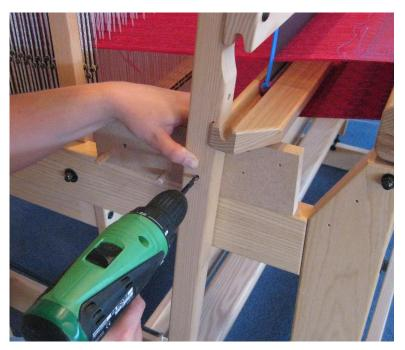
Before you drill completely through the upright, remove the jig and press it against the rear face where the drill will come out, preventing the wood from splinting.
