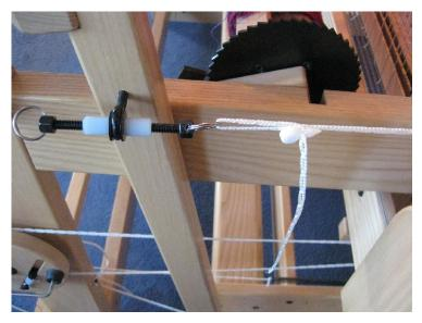
Attach the cord to the eye of the cord connector, using a Texsolv peg as shown in the picture.
