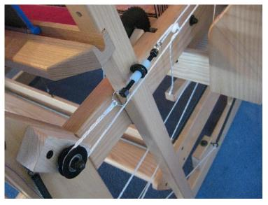
Take the other cord and attach the end to the other eye of the cord connector. Repeat in reverse connection the first cord, over the rollers and attach it to the other connector.
