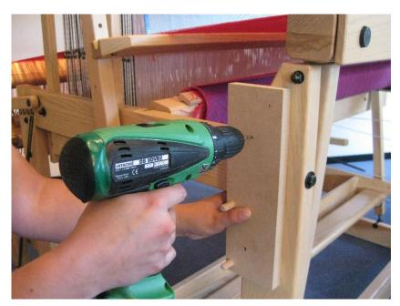
Press the jig against the front post. The dowels help to hold the jig in position.
