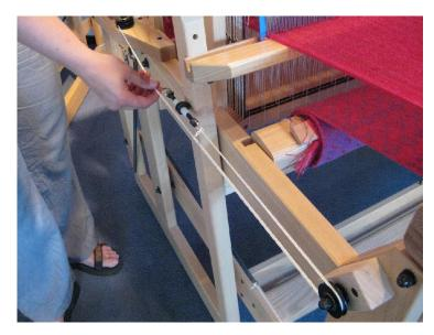
Lead the cord over the roller at the front and than to the back, around the lower roller of the two.
