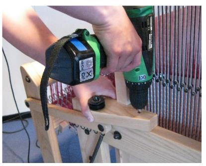
If the drill bit is not long enough, use the block only to drill the start of the holes and then remove the block to drill deeper.
