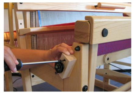
Screw at both sides the blocks with the single roller onto the front posts.
