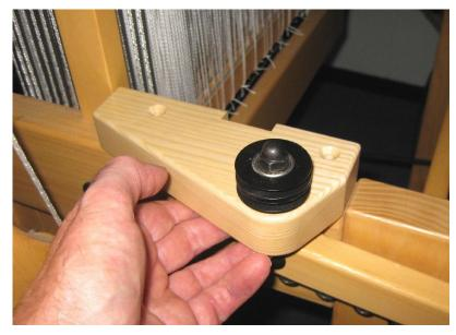
The blocks with the double rollers should be screwed onto the sides of the loom at the rear of the middle section. In this picture, you can see its position on a 16 shafts Megado. On a 32 shafts Megado the upright of the middle section is located into the notch of the roller block, as shown in next picture. This also shows drilling the 3 mm pilot holes.
