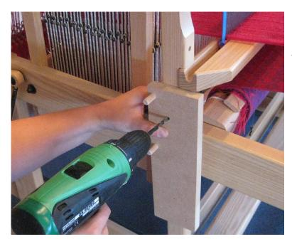
Use the jig to drill the 6 mm hole into the uprights of the beater. Position the jig against the bottom of the beater rail, with the dowels resting against the backside of the upright.
