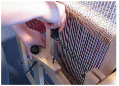
Position the block in place and crew it tight, using a screw in each hole.
