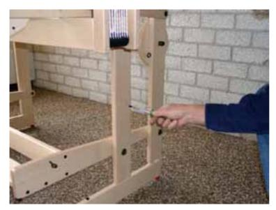
Screw the 4 x 17 mm screw in the upright of the frame until the screw head protrudes approximately 1/4" (5 mm).
