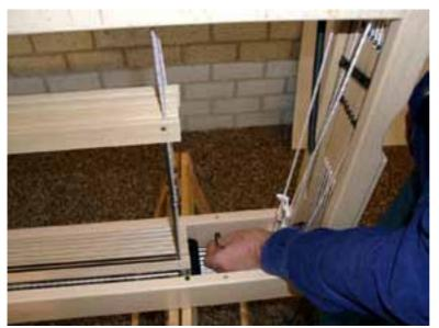
Remove the barrel nuts from two threaded rods and put the barrel nuts in the respective holes where the side rail needs to be mounted to the castle frame.
