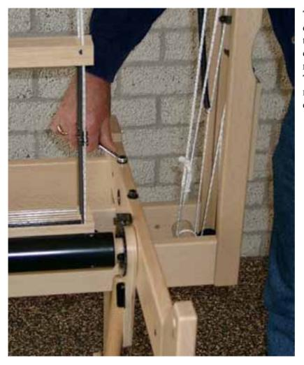
The frame of the Octado is complete and now you have to tighten the cap nuts of the connection between the right side rail and the castle. The sawhorses or table is not required anymore and can be removed.
