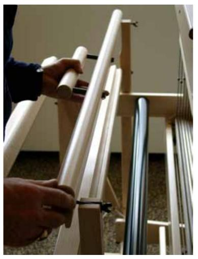
Slide the washers over the carriage bolts and twist the wing nuts a couple of turns onto the carriage bolt. Assemble the upper reed holder to the uprights. Slide the carriage bolt from the top into the slots and insure that the washers rest under the wing nuts and not between the upright and the reed holder. Keep this in mind when you change your afterwards.
