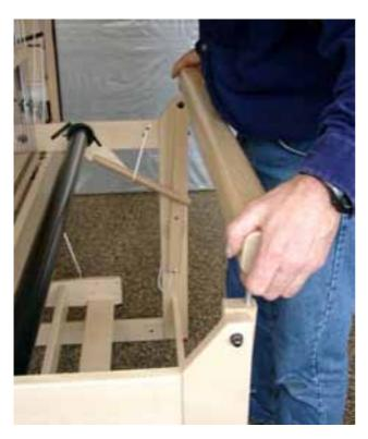
Slide the breast beam onto the pins of the wooden posts; first on the one side partly, and then on the other side.
