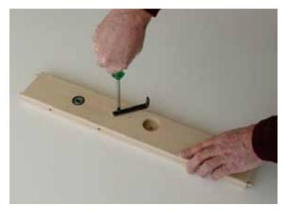
Take the second side rail, marked JD, and screw the large ratchet to it with screw 4.5 x 20 mm. Once tightened, loosen the screw slightly to allow the ratchet to rotate freely.
