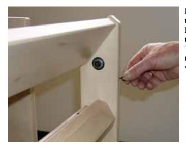
Put the two remaining screw eyes into the uprights of the back beam section. Later on you will attach the cross sticks to these if you warp in that way. This will leave the cross sticks between the warp beam and the back beam, when you advance the cloth.
