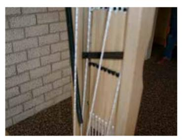
Use the knurled nut of the attachment to the treadle to adjust the height of the dobby knife. The dobby knife is the black metal bar that goes up and down when you turn the knife pulley. In its neutral position, the dobby knife should be high enough that the screw head of the last dobby hook can move freely below it if the dobby hook is pushed forward. Leave about 1/4" (5 mm) clearance.
