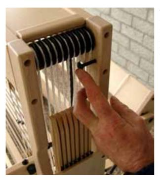
The dobby hooks are located between two uprights. The rear upright has two holes in it for the support of the dobby head. Put a carriage bolt from the inside through the top hole. You need to lift the cords one by one over the head of the carriage bolt.
