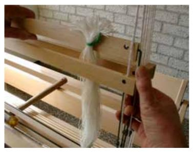
Push the dobby hook at the side of the castle inward. This will unlock the shaft, and you can pull the shaft up.
