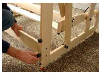
Screw the two buffers into two of the four holes in the front of the right hand upright. Depending on the chosen height of the foot rail, this will be the first and the third hole, or the second and the fourth hole measured from the bottom.
