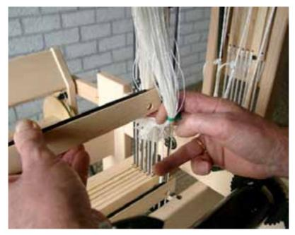
Slide the bundle of heddles over the shaft bar. The heddles still have the lower two twist ties attached.
