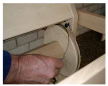
Position the large eye of the brake cable over the end of the carriage bolt and guide the cable one turn around the brake disk.
