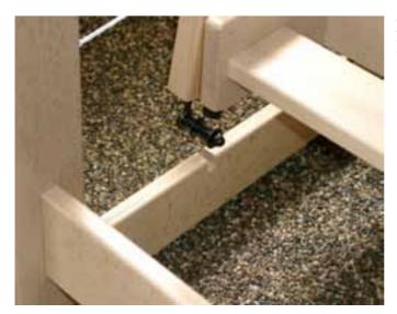
Put the hinges into the openings in the lower side rails.
