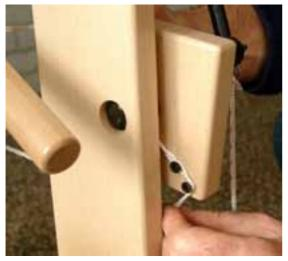
Attach the cord in the same way to the two screws on the lower point of the reversing disk. Remove the cord from one or two pulleys; this will give you some slack, which you will need to attach the cord. Put the cord back over the pulleys.
