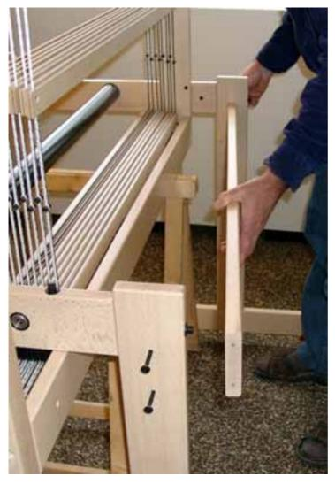
Put the 4 screws 5 x 50 mm in the holes of both rear uprights.
