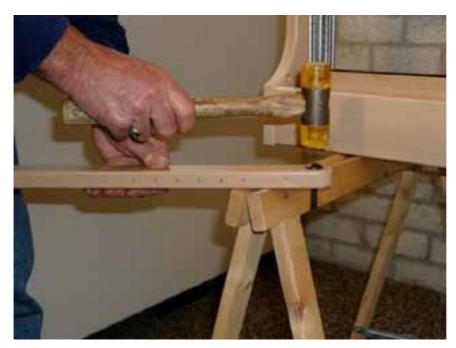
Take a hinged arm out of Box B and install a carriage bolt into it. Refer to the diagram to see where the row with small holes is in relationship to the carriage bolt.
