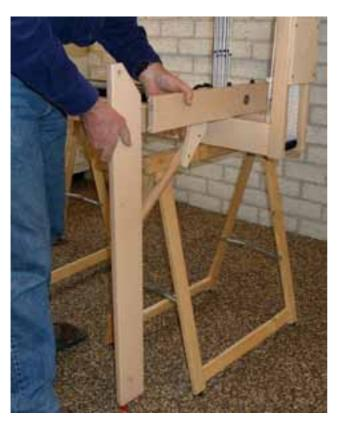
Make the J-J connection: Slide the upright onto the wooden pins (dowels) of the right side rail.
