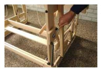
Next you slide the reversing disk onto the carriage bolt and tighten the cap nut.
