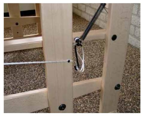
You should hang the hook on the screw eye when not in use, otherwise it can damage the wood when the back beam section goes up and down.
