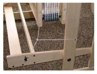
Attach the end of the first cord, again with the hook, to the eye of the treadle.
