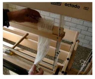
Remove the two twist ties that keep the upper part of heddles together.
