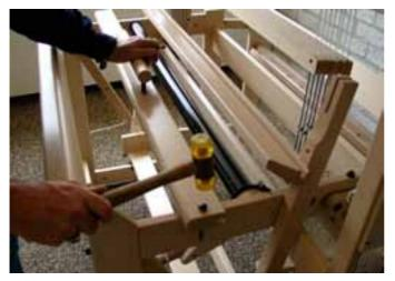
Tap the carriage bolts into the holes at the end of the upper reed holder. Support the reed holder by putting it on the side rails of the loom. Make sure that the handle is facing up.
