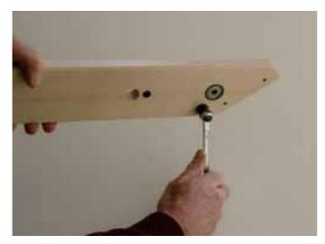
The right hand vertical post has a hole for the longer shaft of the warp beam to go through. Attach to this vertical post the attachment bolt for the brake cable: Insert the carriage bolt m6 x 40 mm into the hole near the ball bearings, so that it protrudes at the side where the black nylon bearing is situated besides the hole for the warp beam axle. Slip on a washer, the piece of nylon tube that will center the spacer bushing, slip on that bushing, the second washer and tighten the cap nut.
