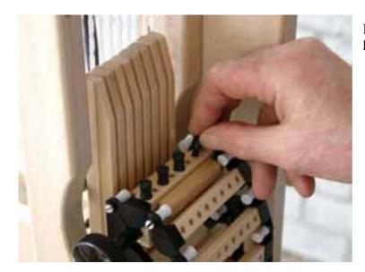
Put four black pegs in alternating holes on the first selection bar.
