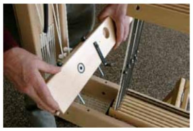
Insert the 2 threaded rods, with washers and cap nuts, from the top, through the holes in the small side of the right side rail. Assemble the side rail to the castle frame by screwing the threaded rods with cap nuts into the barrel nuts. Do not tighten the nuts. The side rail still needs to be loose.
