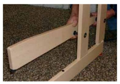
Attach the treadle sides by placing the ends of the carriage bolts through the ball bearings from the inside of the uprights. Put the cap nuts on the bolts and tighten with the 13 mm wrench. Both treadle sides are installed this way.
