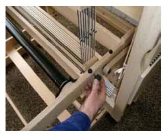
Turn the black buffers into the top hole in the side rails of the loom.
