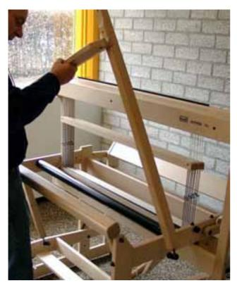
Turn the vertical hinges into the bottom of the uprights. By turning these hinges in and out, you can adjust the height of the reed exactly after threading through your first warp.
