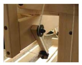
Guide the anchor cord from the top of the reversing disk behind the upright of the beater to the angled guide block with the pulleys. This cord needs to go around the higher of the two lower pulleys and than over the third pulley and up.
