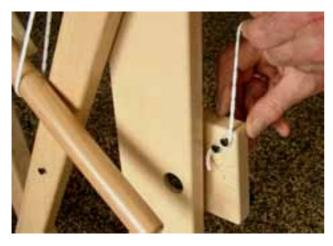
When you keep the brace of the reversing disk horizontal, you will find at the back two screws at the top and bottom point. These screws are to connect the cords of the anchor.
