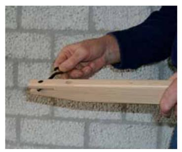
Place the barrel nut into the hole of the brake pedal and turn the threaded hook so far into the nut, that the threaded end sticks about 1-3/4" (2 cm) through.
