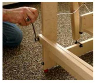
Place a small washer and then the 22 mm spacer bushing onto the lag bolt. Put the bolt through the hole at the other end of the treadle and slide the large washer around the lag bolt. Watch out that the head of the lag bolt sits on the same side as the screw you just installed.
