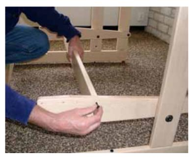
We now connect the treadle sides by installing the two remaining rails between them with the 5 x 50 mm screws.
