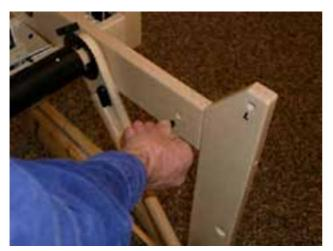
Insert a barrel nut into the side rail.
