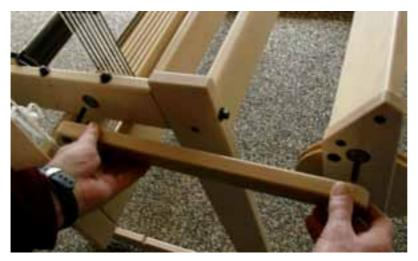
Slide the large washers and then the two smaller washers onto both carriage bolts. Slide the bolts, through the ball bearings of the side rail and at the same time through the ball bearings of the right upright of the back part.
