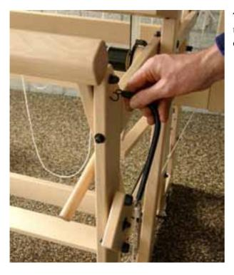
Turn the screw hook into the top of the upright and attach the spring of the reversing disk to it.
