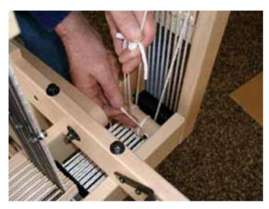
Turn the knife pulley slightly by pulling on the cords and hook the end of the longest of the two Texsov cords around the screw head on the knife pulley.
