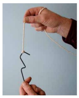
The bent piece of steel wire in the hardware bag is the anchor. The anchor will pull the dobby roller a quarter turn every time you depress the dobby treadle.
