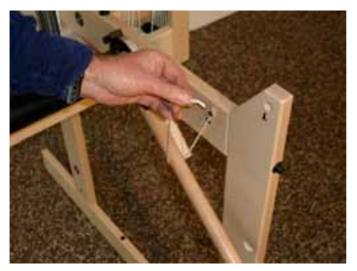
Take the last screw out of the hardware bag, install it in the hole in the right side rail, and leave the head of the screw protruding approx 1/4" (5 mm).
