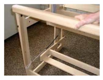
By connecting the cords of the springs to the screws on the spring arms, you make the breast beam movable. You will use this system later to regulate the warp tension.
