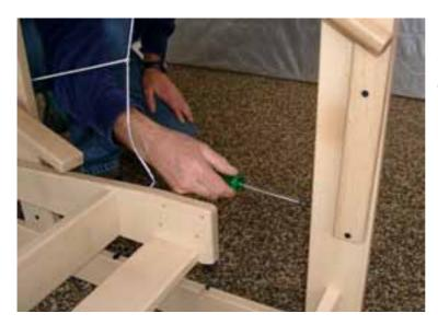
Put two screws in each wooden post and one in the back of the upright.
