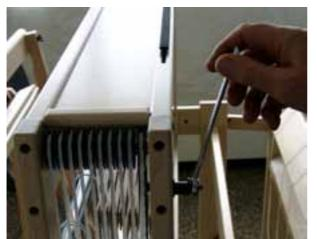
Slide a washer, the 12 mm spacer bushing and another washer over the end of the carriage bolt. Tighten the nut until the square part of the bolt, just under the head of the bolt, pulls completely into the wood. Remove the nut, washers and spacer bushing from the bolt again. Do the same with the other carriage bolt in the lower hole. This hole is located behind the dobby hook guide plate.
