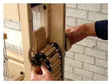
Turn the top of the dobby roller towards the top of the loom. Guide the first selection bar between the guide disks. These are two washers, situated just below the dobby roller on the mounting board.
