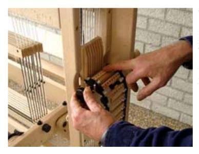
Take the assembled chain of selection bars and put the first one in the groove on top of the dobby roller.
