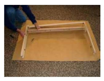
Insert the long shaft of the warp beam through the right upright and slide the left upright onto the short shaft on the other side of the warp beam.
