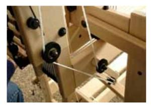
Guide the cord around the pulley, over the lower pulley of the angled guide block and to the reversing disk.
