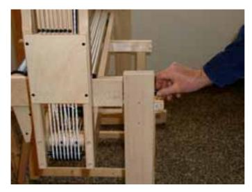
Assemble the rear uprights and lower side rails on both sides of the loom (Connections D-D, F-F, C-C and E-E). First slide the wooden parts over the dowels and than make the connections with the threaded rods, barrel nuts washers and cap nuts.
