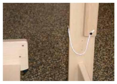
Connect the lower two screws on both sides of the loom with a cord.
