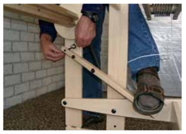
Put the eye on the other end of the brake cable over the hook of the brake pedal while you push the brake pedal down.
