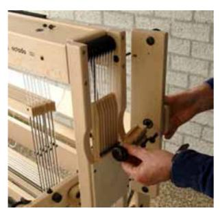
Slide the dobby mechanism over the carriage bolts, slip on the washers and tighten it with the nuts.
