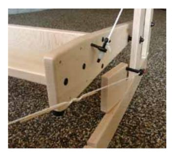
In the neutral position there is about 1/4" (5-8 mm) space between the locking block and depressed treadle.
