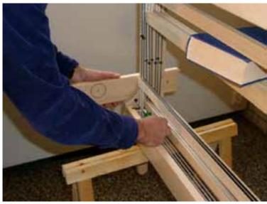
During the assembly of this side rail you need to lift up the first two shafts in order to be able to access the screw hole in the front.
