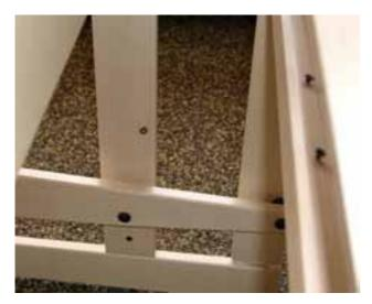
Put two of the screw eyes in the appropriate holes in the sides of the loom, and hook the springs onto these eyes.
