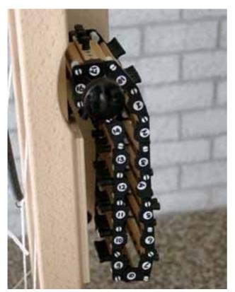
Slide the spring to one end of the brace. With the dobby treadle you can turn the dobby roller a quarter turn. If you put the spring on the other end of the brace, the dobby roller will turn in the other direction. By reversing direction, you can weave your programmed pattern in mirror image; i.e. weave forward or backwards.
