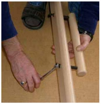
Assemble the handle to the upper reed holder: Slide a washer over the lag bolts and then put them through the holes in the upper reed holder.
