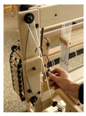
The cord has to go over the highest pulley on the dobby head. The anchor needs to be attached to two of the four rollers that are on the back of the wooden knob on the dobby roller.
