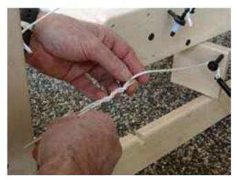
Fine adjustment can be made with one of the wooden pins. When you put a wooden pin zigzag'd through the Texsolv cord, the cord will shorten 1/8" (3mm) for every two holes the pin goes through.
