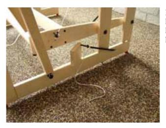
Put the shaft of the locking block in the hole of the lower side rail. Put a screw hook further back onto the side rail and hook the spring around it.
