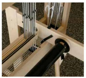
Install the cloth beam with the wooden end into the hole of the right side rail and the metal end into the circular groove of the left side rail. Be sure that the big ratchet is turned in the backward position.
