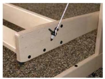
Put the plastic hook with washer and knurled nut through the eye of the treadle and attach the second hole of the cord to the hook (Do not count the hole where the cord is cut).
