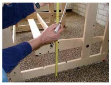
Use a black felt tipped marker to mark the hole in the cord that is 19 1/4" (49 cm) above the floor and remove the cord from the plastic hook again.
