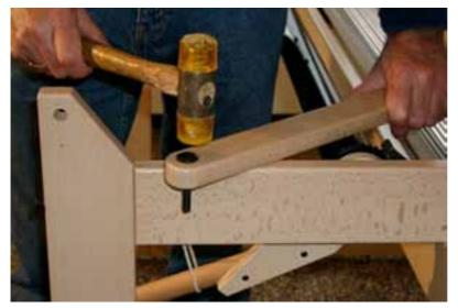
Install the remaining two carriage bolts from hardware bag # 1 onto the other hinged arm. Pay particular attention to the position of the small holes; the hinged arms need to be mounted opposite to one another, (in mirror image to each other)
