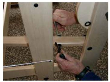
Take the threaded eye and remove a nut and one washer.
