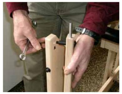
Slide the large washer and spacer bushing, over the carriage bolt and attach the wooden posts to the front uprights of the loom. Make sure to connect K-K and L-L. This determines left and right. Use the small washers and cap nuts to finish the assembly.
