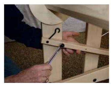
Slide the brake pedal over the spacer bushing onto the carriage bolt, than the small washer and the cap nut. Tighten the cap nut well.
