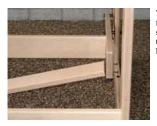
The other rail is mend to push the treadle to the floor. There are three sets of holes in the treadle sides. These holes can be used to adjust the treadle in three positions, depending on the length of your legs.
