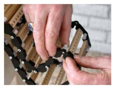
Connecting the first to the last selection bar requires a bit of skill. The hinges of the connecting links, left and right, need to be pushed together at the same time.
