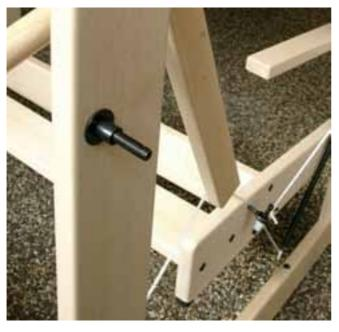
Put the carriage bolt of the reversing disk through the hole in the right hand upright. Slide the large washer onto the bolt and than the ½" (12 mm) spacer bushing.
