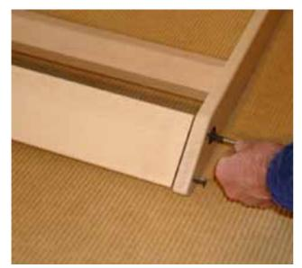
Also attach this upright to the back beam with two screws 5 x 50 mm.
