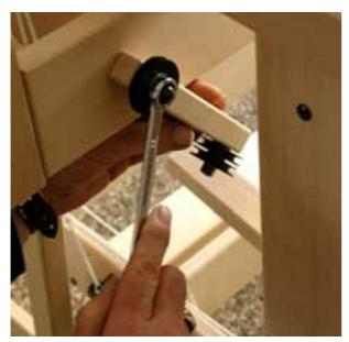
Take the guide block with three pulleys and disassemble the carriage bolt with one pulley. Put the carriage bolt from the inside through the lower back rail of the castle. Slide the guide block, the two washers and the pulley onto the carriage bolt. Tighten the cap nut while the guide block points in about the same direction as on the picture.
