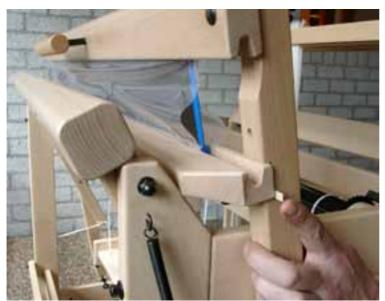
The upright that leaves the buffer latest when you pull the beater, is the one that needs one or more cardboard strips in its slit connection with the lower reed holder.
