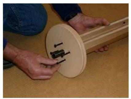
Slide the brake disk onto the longest one of the protruding shaft of the warp beam; the sides marked Q must face each other.
