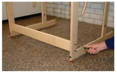
In the same way install the foot rail on the front of the loom, between the front uprights.
