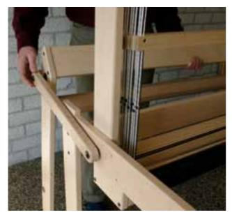
Put a carriage bolt through the hole in the hinged arm that is connected to the left side rail. First slide the large washer and then the two small washers onto the carriage bolt.
