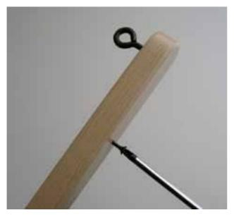
Put the 4 x 17 mm screw in the other side. The head of the screw should protrude 3/16" (5 mm) out of the wood.
