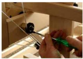
Adjust the angle of the three-pulley guide block. The two cords need to run parallel to the guide block. Lock the guide block in this position by screwing the remaining 4 x 30 mm screw into the guide block.
