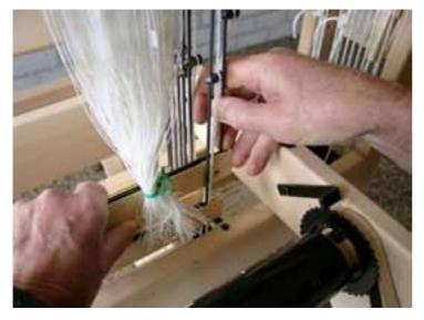
Pull the lower shaft end out of the lower shaft bar.
