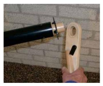
Slide the cloth advance lever (from box B) onto the cloth beam (from box C) and make sure that the ratchet is on the right side of the ratchet wheel.
