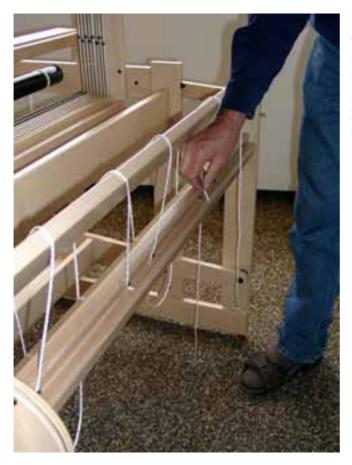
Hook the end of the tie-up cords around the screw heads of both, cloth beam and warp beam. Hardware bag 6 is the same for both Octado 90 (36") and Octado 110 (44"). So with the Octado 90, you will have two extra tie-up cords, which will not be used.
