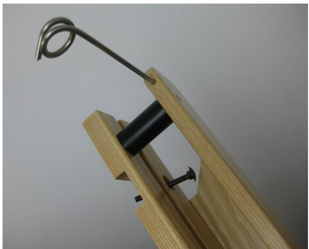
Insert a bolt through the hole at the inside of the catch box.
