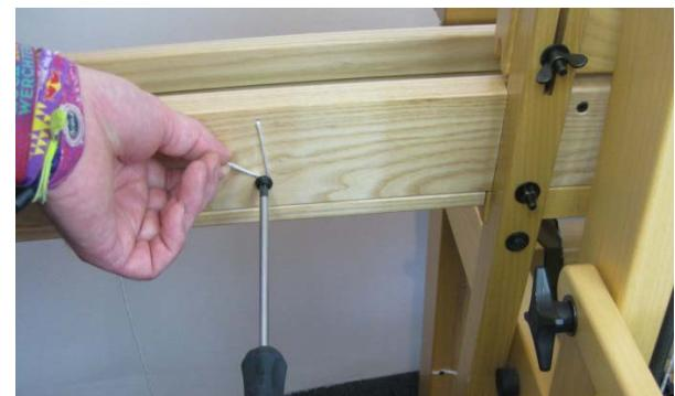
The correct clamping of the shuttle in the catch box can be adjusted by adjusting the length of the piece of cord between the slide block and the screw head.
