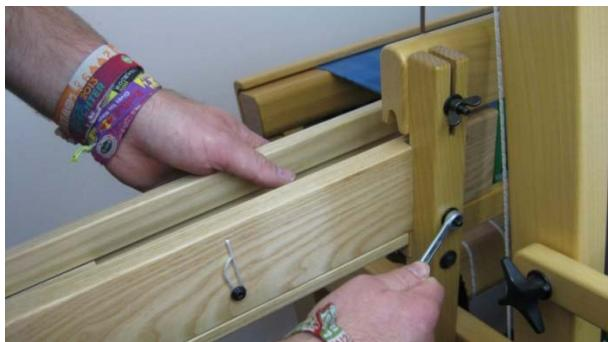
Slide a washer over the protruding end of the bolt and fix the assembly by fastening the nut.
