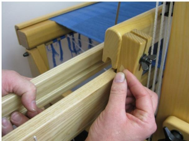
If necessary, adjust the notch of the catch box on the beater upright using thin spacer strips to get a snug fit.
