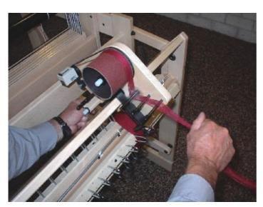
Initially, the threads do not need to be exactly side-by-side on the friction drum. However, if you need extra room, pull the warp a couple of times back and forth. This will position the threads neatly side by side.
