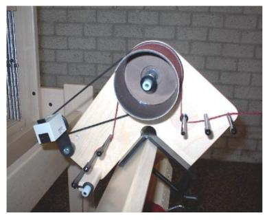
Attach the tension regulator on the back beam, just above the section you want to fill.
