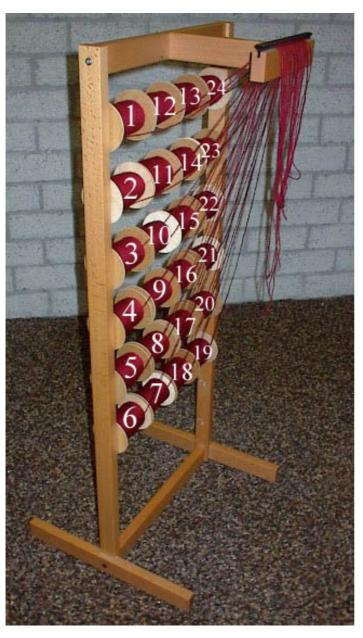
Hang the shafts filled with Bobbins in the Bobbin Rack. The thread has to run from the bottom of the Bobbin to the Raddle. Position each thread in an opening of the raddle. In the picture we have numbered the Bobbins. This shows the sequence of the threads in the Raddle.
