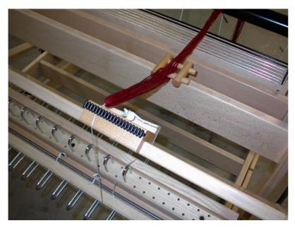
Lead the warp chain through the loom and over the breast beam. Advance the warp beam so that the end of the warp comes close to the back beam.
