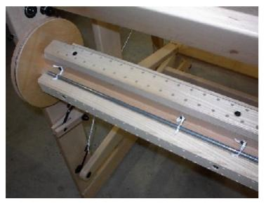
Hook the steel tie-up bar with the Texsolv cords to the screw heads of the warp beam.
