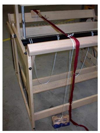
Use the cord to attach a weight to the warp hanging just above the floor. This weight determines the warp tension on the warp beam. So for each section you have to use exactly the same weight.
