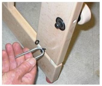
Use a clip of the sectional warping to tighten the screw eyes into the bottom of the uprights of the back part.
