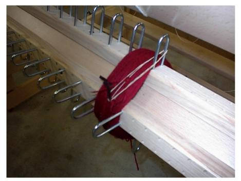
Attach the end of the warp with an elastic band to a section clip. Don't use a clip of a section that still has to be warped.
