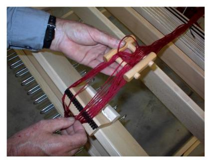
Take the cross holder with the warp in one hand and divide the warp yarns in the raddle. The raddle has 2 openings per cm or 5 per inch.
