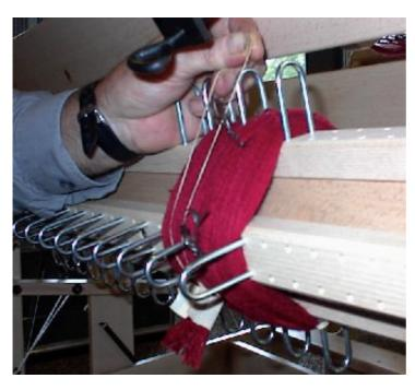
Attach the end of the warp with an elastic band to a section clip. Don't use a clip of a section that still have to be warped.
