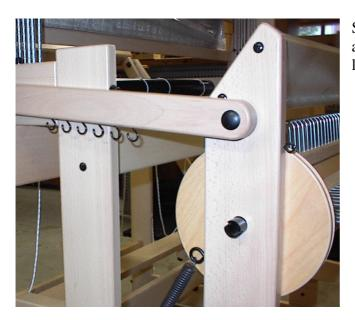
Screw six hooks on the bottom of both hinge arms, with there opening facing the front of the loom.
