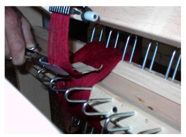
When the desired warp length has been beamed-up, you can use a piece of tape to keep the warp yarns in proper sequence. This is necessary, because there is no cross in the warp. The sequence of warp yarns on the tape is sufficient to keep the yarns in order while bringing the yarns forward and through the heddles. If in this process a couple of yarns are mixed-up, it should not affect the weaving.
