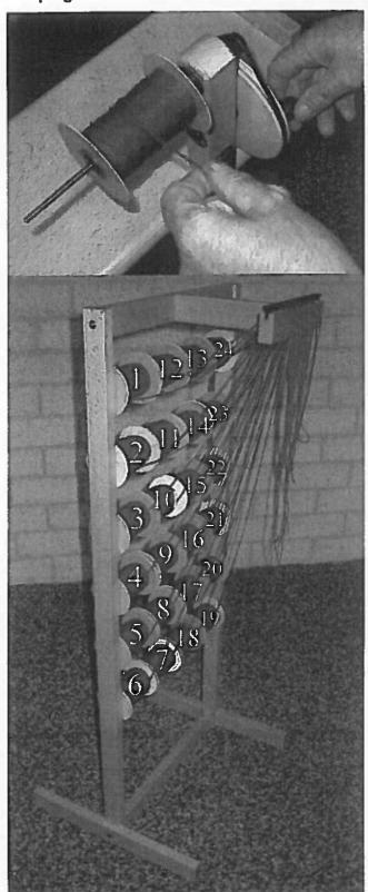
For every thread in the section you need a bobbin on the bobbin rack. With the bobbin rack you can do a maximum of 16 threads per cm on metric beams, or 32 threads per inch on Imperial beams.
