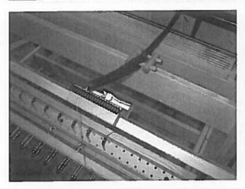
Lead the warp chain through the loom and over the breast beam.
