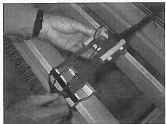
Take the cross holder with the warp in one hand and divide the warp yarns in the raddle. The raddle has 2 openings per cm or 5 per inch.
