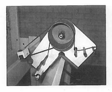
Attach the tension regulator on the back beam, just above the section you want to fill. Before running the threads through the tension regulator, loosen the two knurled nuts till the friction drum turns lightly. Take all but one of the plastic disks from the third shaft.
