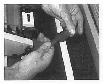
Put a knot in the end of the warp that sticks out of the warp tension regulator.
