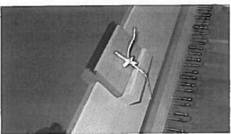
Attach the raddle on the back beam with the Texsolv cord and peg. Fix the raddle in place, above the section you intend to warp by pushing the wedge underneath the Texsolv cord.
