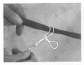
There is a cord included to attach a weight to the warp. At one end it has a double loop. The picture shows how you can attach this loop to the warp chain in a way so that you can easily pull it loose and move it along the warp chain.
