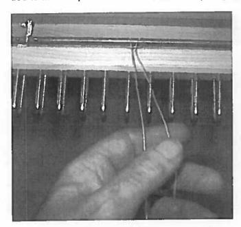
You will find a ball of cotton yarn in the package. With this yarn you can make a loop, a bit longer than you need to go from the warp beam over the back beam to the shafts.
