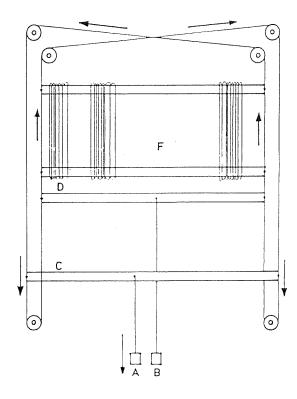
Parallel countermarch system: Each shaft is attached to a cord which goes over all six rollers. The ends of the cord are joined, forming a continuous loop. When treadle A is depressed, the lower lam C, attached to the outside of the loop, moves down, pulling the shaft up. When treadle B is depressed, the upper lam D, attached to the inside of the loop, goes down pulling the shaft with it.
