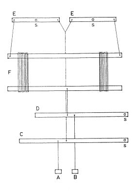
Traditional countermarch system: The points marked S are the pivoting points for the lams C and D and the jacks E. When
