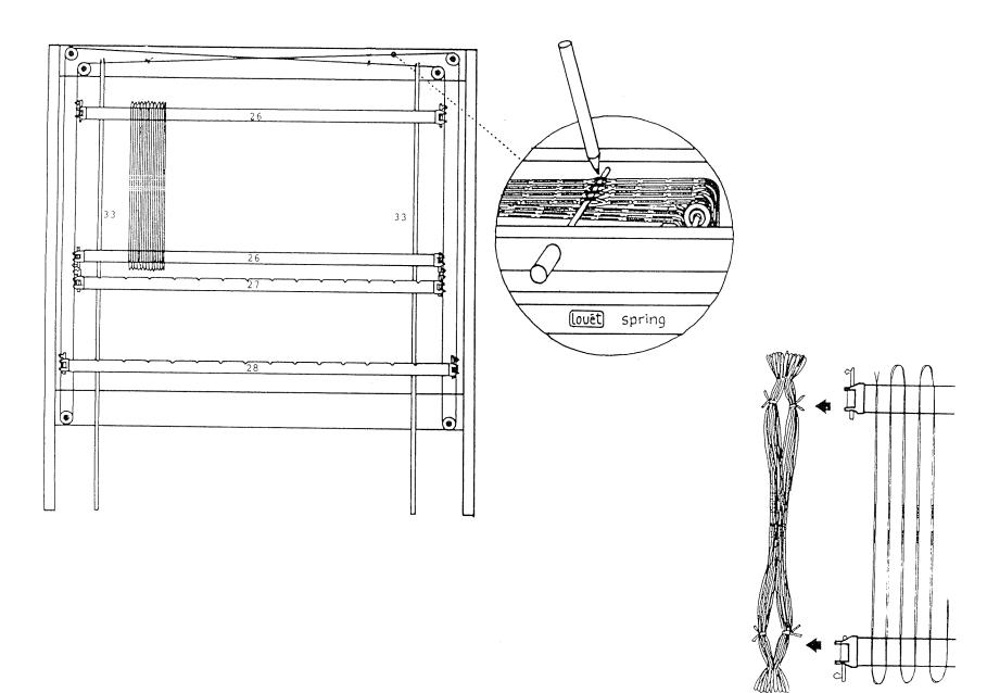
For hanging the shafts and lams, you will need the measuring rods, 33, the bundles of texsolv heddles, the locking pin and a marking pen.
