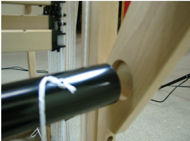
Take the beam support out of the upright to insert the beam into the blind hole.
