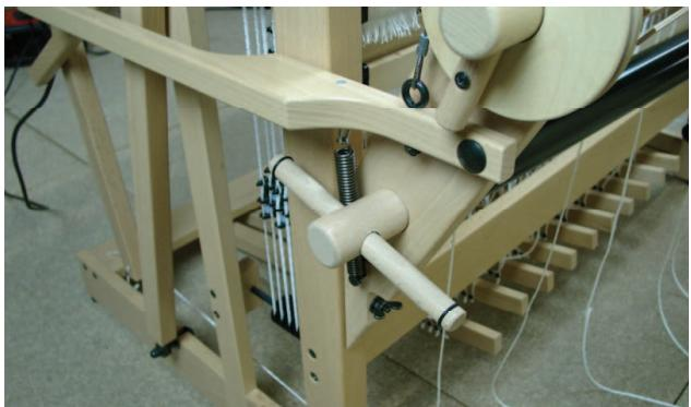
Insert the beam handle through the hole in the beam and secure it by rolling the rubber O-ring into the groove around the handle.
