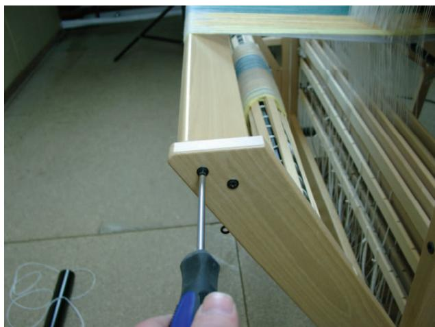
Loosen the connection to the back beam by unscrewing the screws slightly.
