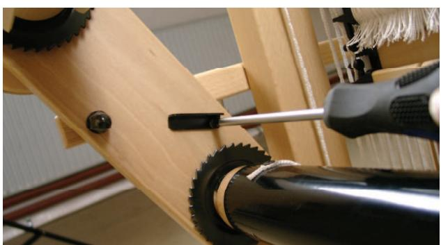
The last little screw is to attach the ratchet. Use the pilot hole close to the ratchet wheel.
