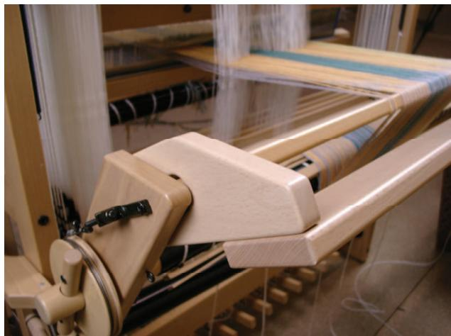
This last picture shows you how to connect both back beams.
