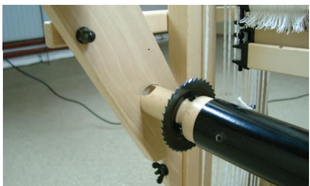
Insert the end of the warp beam into the hole of the beam support at the other side of the loom.
