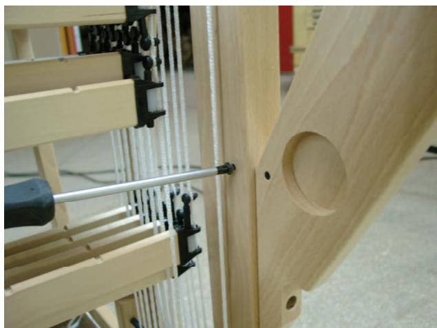
On the inside of the upright, unscrew the polyurethane dowel connection.
