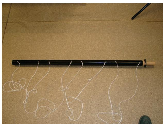
Attach the beam cords to the warp beam.
