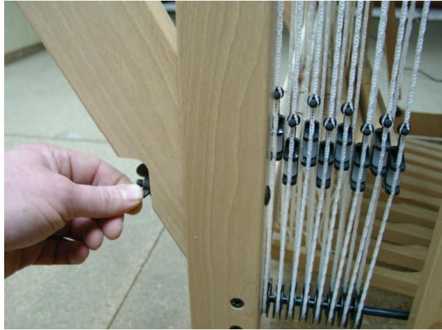
Disassemble the warp beam support at the left upright of the loom by removing the wingnut and pull out the bolt on the backside of the upright.
