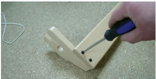
Attach supports for the 2<sup>nd</sup> back beam to the back beam with the 4 remaining screws.
