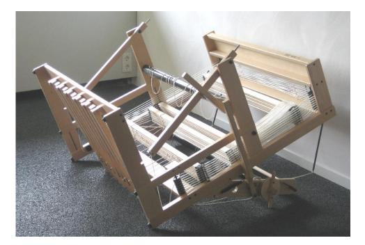
Remove the beater and the breast beam from the loom and place it on its back side.
