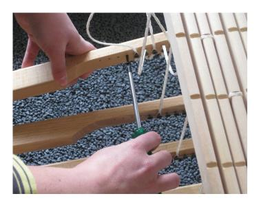
In the same way, screw the small screws into the holes on the existing treadles of the loom. These holes will correspond to the new shafts.
