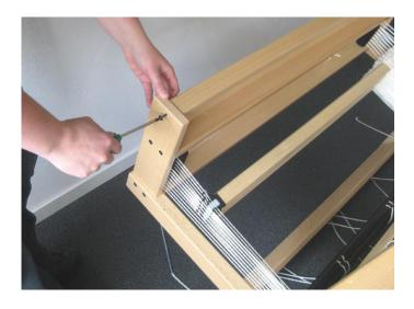
To add the rollers onto the axles at the top, you have to disassemble the two rails that have the shelf in between.
