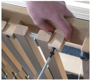
Mount at both sides of the existing treadles two new treadles, using an axle, a nylon spacer, a mounting block and a big screw.
