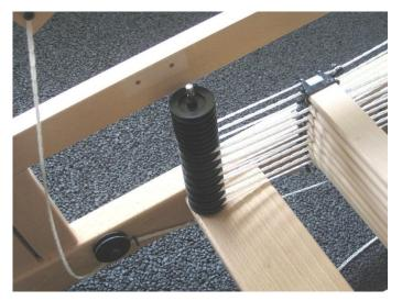
Replace the pieces of nylon tube with 4 rollers at both lower axles.
