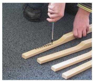
Screw the small screws into the holes of the four new treadles, so far that the screw heads protrude approximately 5 mm (3/16"). The thread of the screws should just disappear into the wood.
