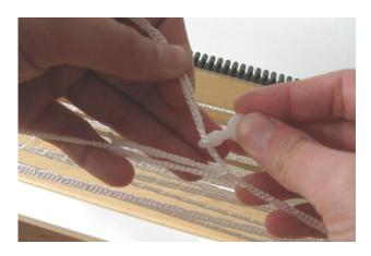
Put the loom on its feet again and lead the new shaft cords over the rollers in the same way as the cords of the existing shafts.
