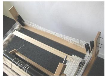
Reassemble the parts after you replaced the nylon tubes with 4 rollers onto the 4 axles.
