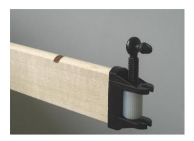
Mount the screw hooks with the knurled nuts onto the shaft bars and lams.
