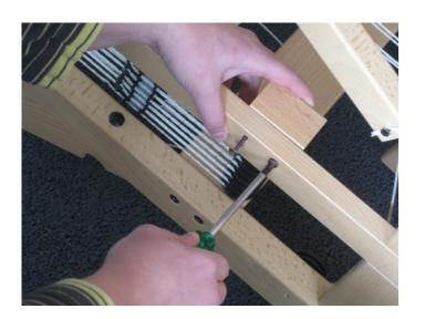
Unscrew the wooden supports at the front side of the lower axles.
