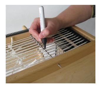
Move the cord connections, alternating left and right and keep them about 20 cm from the rollers. Insert the locking pin through the cord loops of the new cords and mark those loops.
