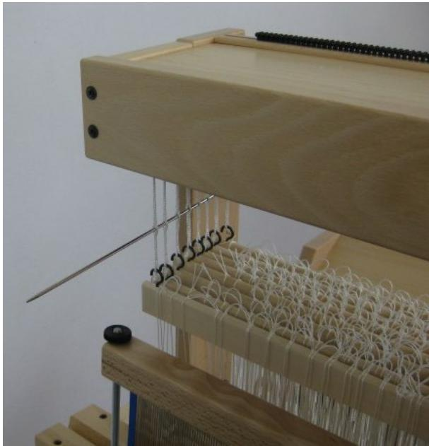
It is handy to insert a knitting needle at the left side through all the cords that the upper shafts bars are connected to. Now when you unhook an upper shaft bar at that side, its cord will stay in place.
