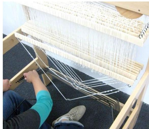
Insert the lams, one by one, with their ends into the nylon bearings, starting with the rear lam:
