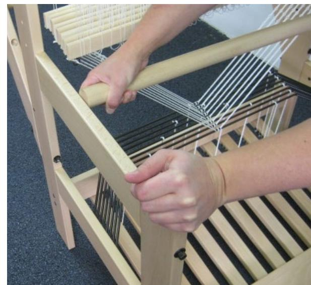
Install the cloth beam in the loom. First insert the side with the ratchet wheel into the hole in the side rail, while you keep the other end of the beam just above the opposite side rail. Because of the beam is slanted in this position, the hole is tight and you have to turn the beam while pushing it through.
