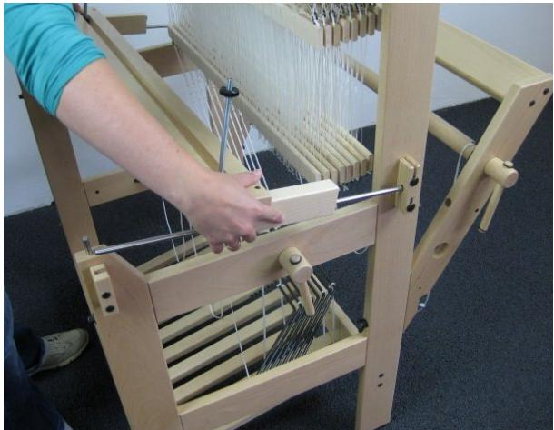
Insert the axles through the bearing blocks at both sides of the reed holder and place the assembly onto the loom. Put the axles into the oval holes first and then at the front, place the ends of the axles into the slots.
