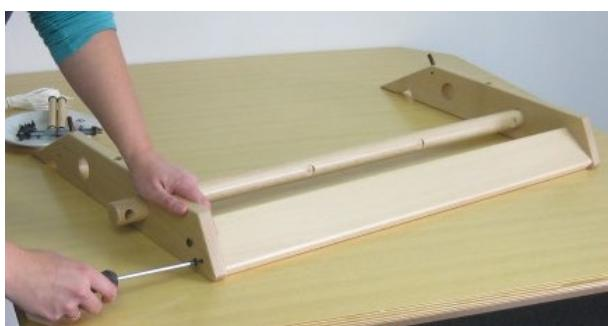
To assemble the back part of the David, use the warp beam supports, the back beam and the warp beam (one of the two round beams with a ratchet wheel).
