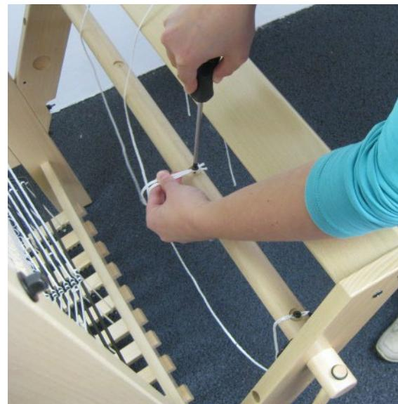
Attach three cords each to the warp beam and the cloth beam with the remaining screws 4x15 mm. Start at one side of the beam with the end of a cord. The other end of that cord has to be fixed together with the end of the next cord in the second hole of the beam etc. Do mind that you fasten the cords in the direction that is locked by the ratchet wheel.
