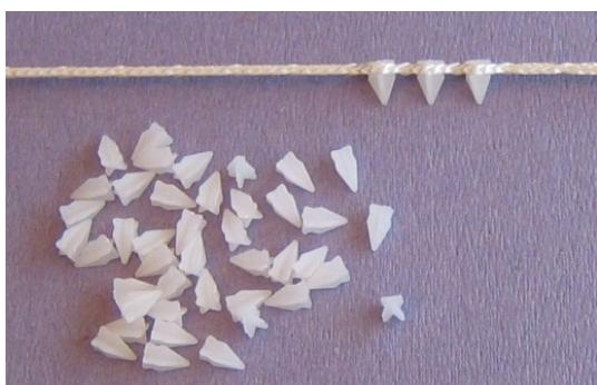
The Texsolv cord is adjustable in length by 12 mm steps (ca.1/2"), according to the loops. For fine adjustment, plastic pegs are used, inserted into the loops of the cord. Each peg through the cord will shorten it about 1.5 mm (1/16").
