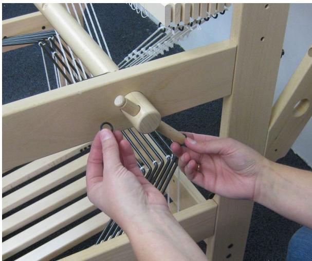
Insert the cloth beam handle through the holes in the cloth beam and secure them by rolling the rubber O-ring into the groove around the handle. A spare O-ring is in the hardware bag extra.
