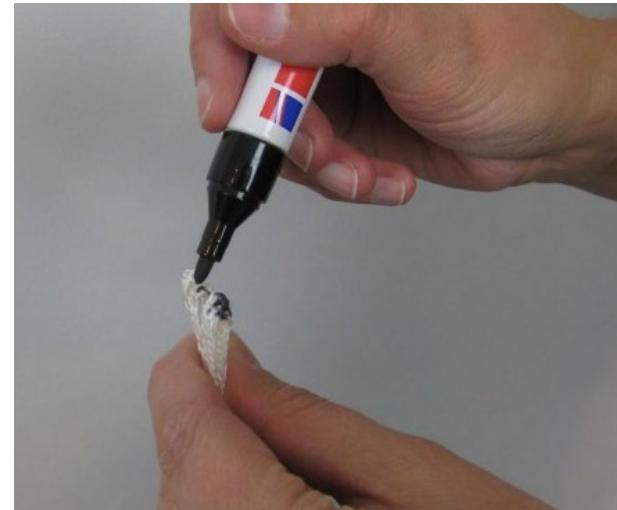
Use a felt pen to mark the center of the beam cords.
