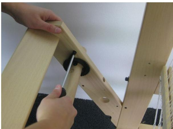
Install a ratchet next to the ratchet wheels of both beams. Use the round head screws 4.5 X 17 mm. Tighten them and then unscrew them just far enough that they can turn freely.
