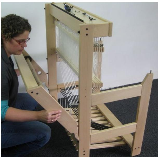
Place the back part in its location by inserting the polyurethane dowels into the holes at the rear of the loom.
