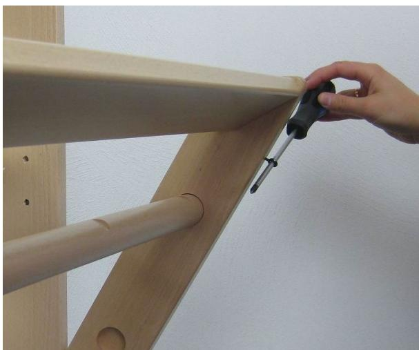
Screw the little screw eyes into the warp beam supports. Use a screw or something similar to twist it easily.
