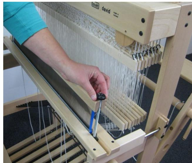
Position the reed and the upper reed holder in between the threaded rods and fasten the assembly with the knurled nuts.
