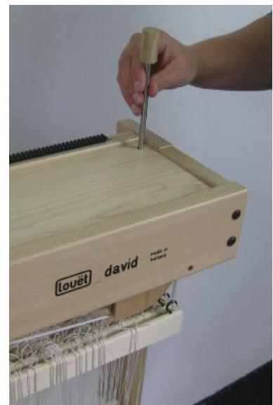
Install the shelf, locating the hole at the right back side. Slide it into the groove at the back rail and let it rest on the dowels of the front rail. The hole in the shelf is meant to store the locking pin.
