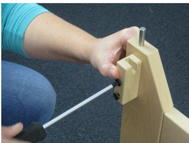
Screw the other two support blocks, each with two screws 5 x 50 mm, on the outside of the front posts of the David. Note the direction of the slot.
