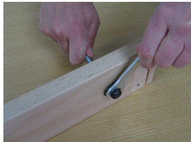
Remove the cap nut and the washer from the threaded end. Insert the threaded end through the hole in the groove of the lower reed holder. The barrel nut fits in the groove and the short end of it should be at the side where the reed will be.
