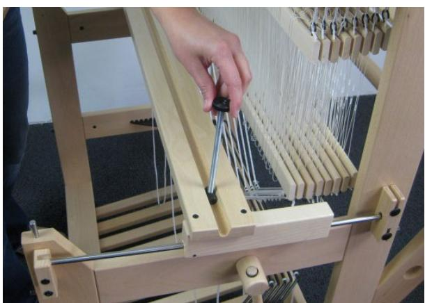
Remove the knurled nut from the threaded ends.
