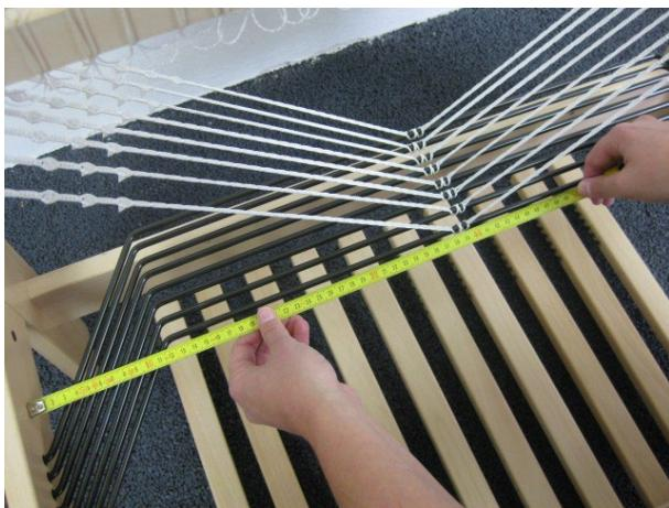
Check the position of the cords that connect the lams to the lower shaft bars. The location on the lams should be exactly in the middle. Replace the connection to the lams if necessary. Start with the ones in the front and the back, so the ones in between can be placed in line.
