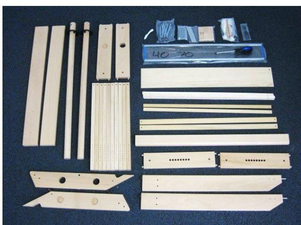
The picture above shows the parts of the David 70 loom. Into each of the lower side rails, eight nylon bearings for the lams are inserted.
