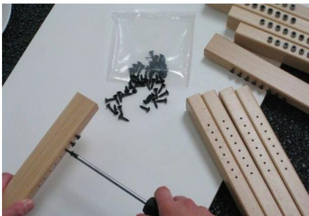
Screw the small screws into the eight holes of each treadle, so far that the screw heads protrude approximately 5 mm (3/16") from the wood. The thread of the screws should just disappear into the wood.
