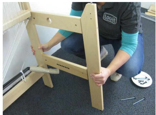
The lower side rails should be mounted the same way, their nylon bearings facing the middle of the loom. After you mounted all four side rails to the castle section, position the front posts onto the dowels of the side rails.
