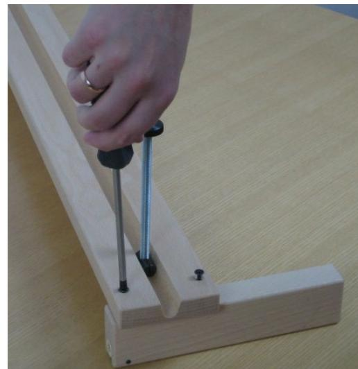
The picture at the left shows in what position the bearing blocks have to be connected to the reed holder. Note the direction of the slope of the notch. Assemble the blocks and the reed holder with the screws 4 x 40 mm.
