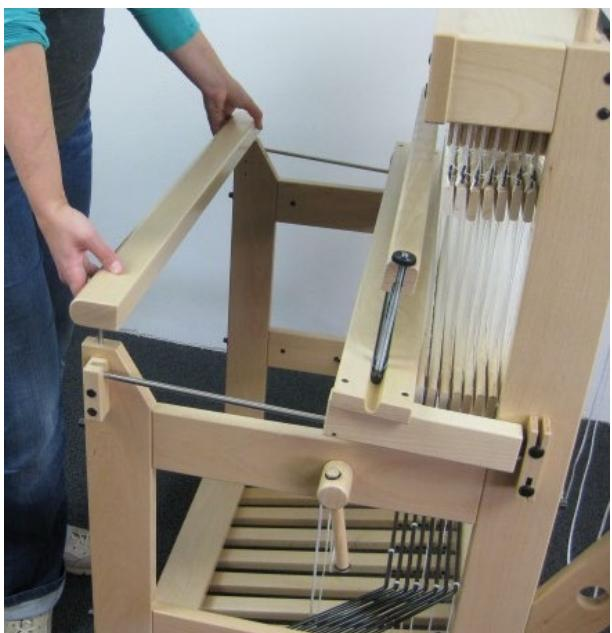
Install the breast beam. The metal dowels on the front posts will fit in the holes of the beam.
