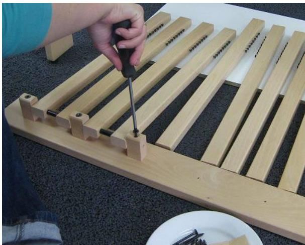
Assemble the treadles onto the foot rail. The screw heads on the treadles should point towards the middle so that the five treadles on the left side are opposite to the five treadles at the right side.
