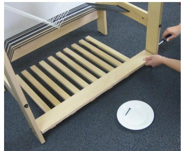
Put the foot rail with the treadles in between the front posts of the loom and connect these parts with the four remaining screws: Connect the foot rail at one side by screwing it on only a few turns, then screw on the other side of the rail completely and finally tighten the first two screws.
