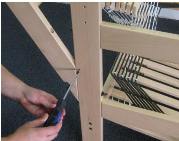
With the two screws 3 X 20 (not the round head 4.5 X 17 ones) you will secure the polyurethane dowels. Left and right upright are the same, so the screw hole in the right leg is on the inside.
