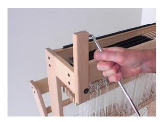
Remove the hanging beater from the loom by pulling the hanger out of the nylon bearing while moving the beater up and down.
