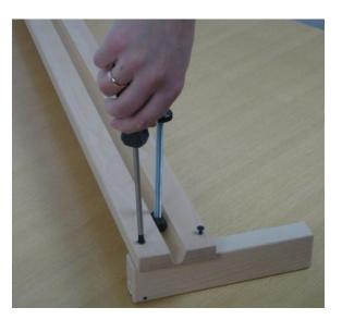
The picture at the left shows in what position the bearing blocks have to be connected to the reed holder. Note the direction of the slope of the notch. Assemble the blocks and the reed holder with the four screws  $4 \times 40$  mm.
