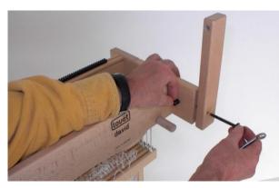
You can also remove the wooden blocks on the front of the loom, they are not necessary anymore.
