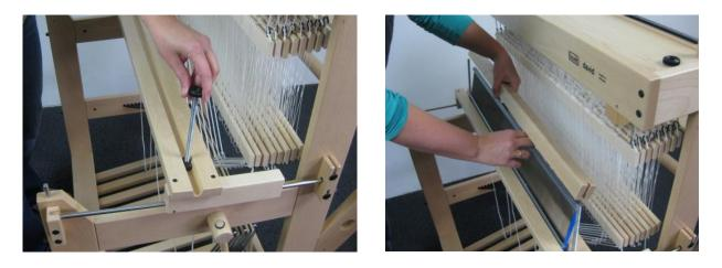
Remove the knurled nut from the threaded ends. Position the reed and the upper reed holder in between the threaded rods.
