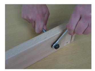
Fasten the cap nut with washer onto the thread that protrudes from the bottom side.
