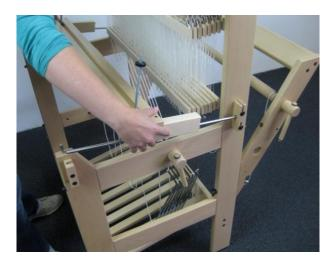
Insert the axles through the bearing blocks at both sides of the reed holder and place the assembly onto the loom. Put the axles first into the oval holes and then in the slots at the front.
