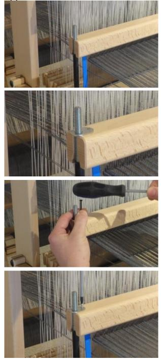
Move the beater a bit forward and remove the knob from the threaded end.
