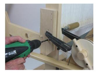
The jig has two dowels that protrude at both sides, so you can use the jig mirror wise at both sides of the loom.
