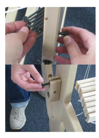
Insert a carriage bolt through the lower hole that you drilled into the main post, place the washer on the end and screw on the wing nut a few turns.
