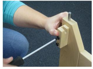
Screw the other two support blocks, each with two screws  $5 \times 50$  mm, on the outside of the front posts of the David. Note the direction of the slot.
